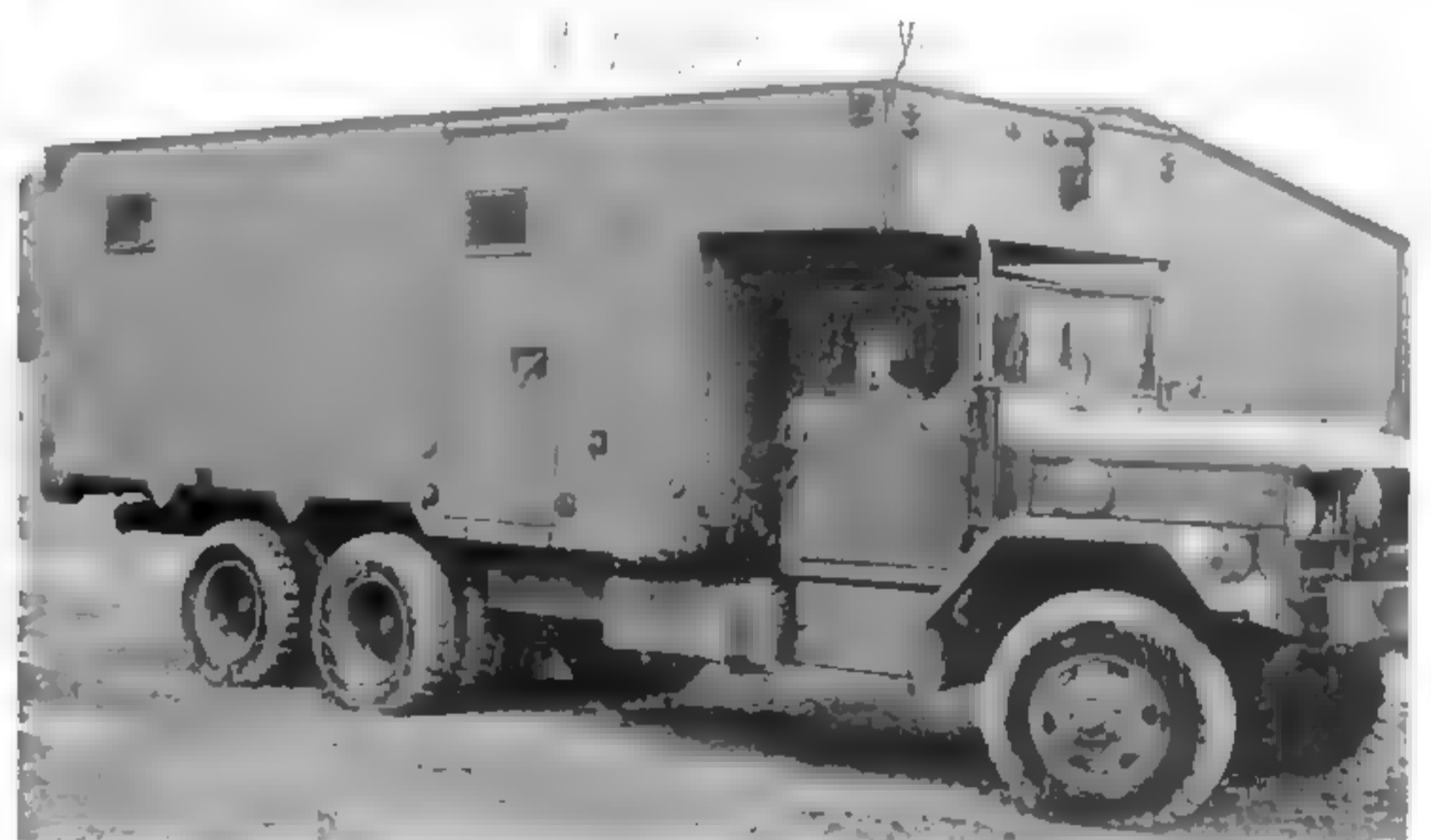
The 3,000-gallon-per-hour purification units were mounted on M46-type chassis. Shown here is one such unit mounted on an M46A2C chassis. (Photo courtesy of TacticalTruck.com)
